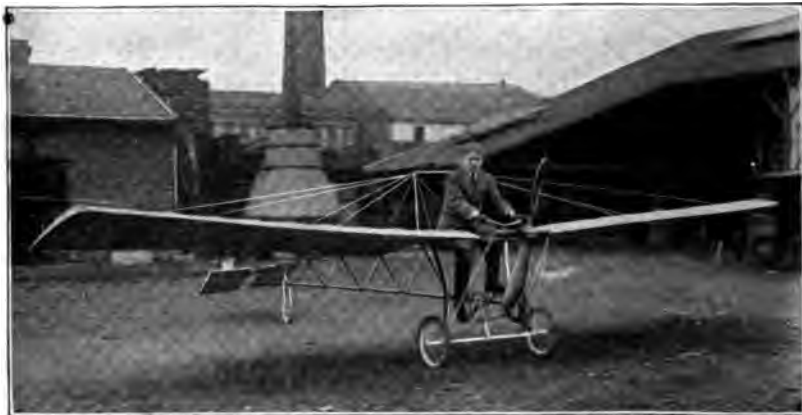
Fig. 38. Aerocycle with Treadle Power for Practice Work
